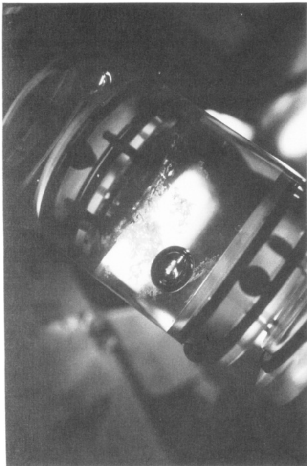
Figure 1. Photograph of nucleation of lead(II) iodide crystals in space and apparatus.
